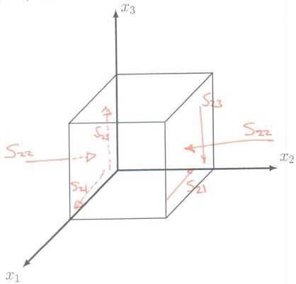
On the figure, correctly indicate (with hand-drawn arrows) the stress components  $S_{22}$ ,  $S_{21}$ , and  $S_{23}$  on both sides of the cube where they act. Use a "compression positive" sign convention.
